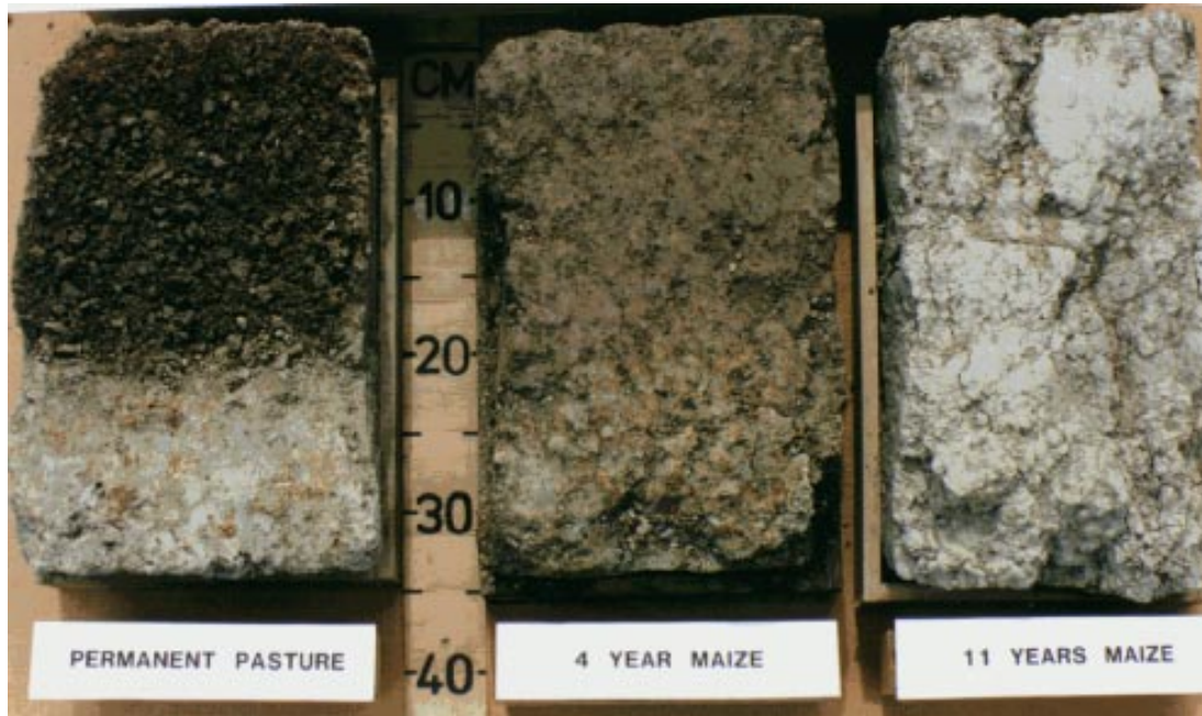
Figure 3: Soil structure can be vulnerable to continuous cropping. This example of a silt loam in the Manawatu District demonstrates the impact of 11 years of continuous cropping for maize on both soil structure and soil organic matter.(Shepherd 1991)
