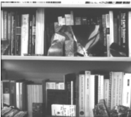
Figure 3 Spectral Target within Field-of-View: Reflection of the overhead light is visible in the crystal in the centre of the frame.
