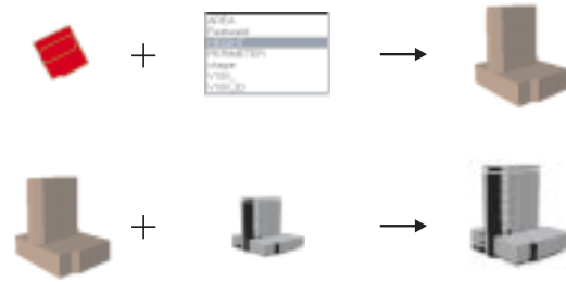
Figure 8. Creation of 2_D geometries from 2D geometries and an attribute value (top), and adjusting a CAD object's scale to match the generated 2_D model (bottom).
