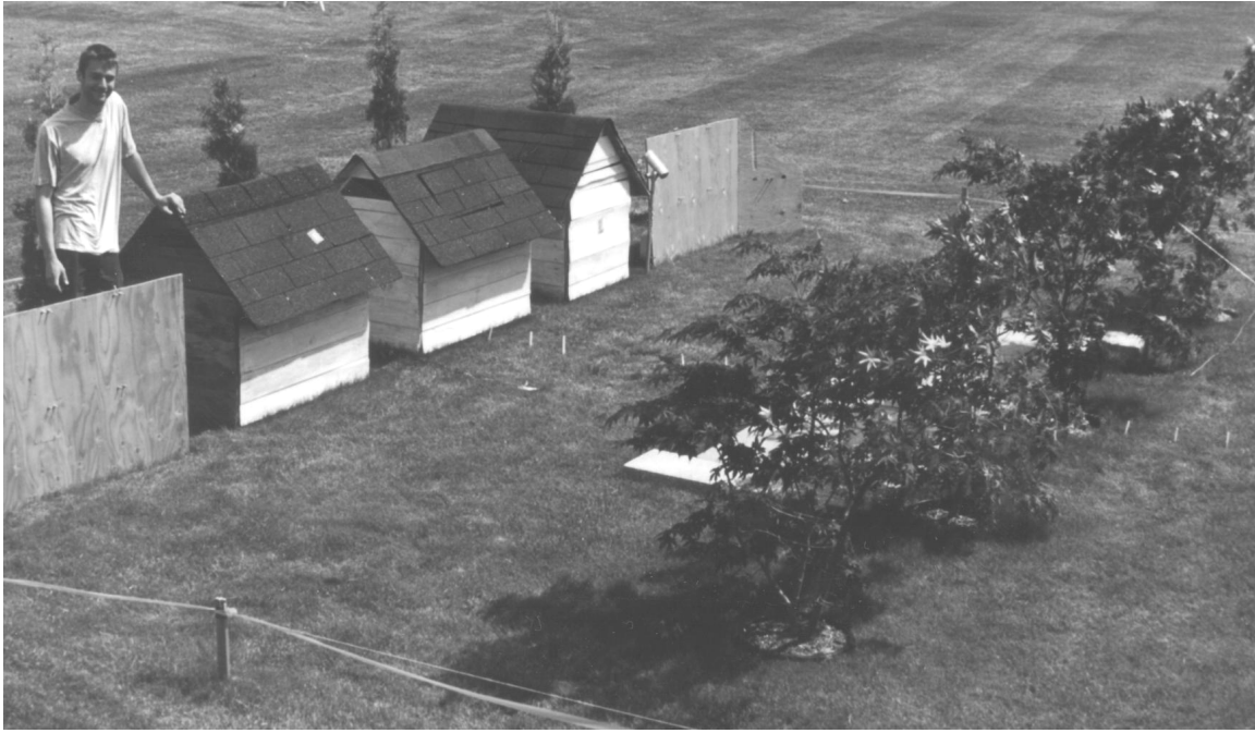
Figure 1: The 1/8-scale urban model run at the University of British Columbia, Vancouver to study urban dew.
