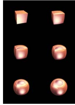
Figure 3: sequence of changes to the twenty-four surfaces that describe both the original cube and the sphere showing the cube tending towards the sphere. The imperfections to the surface of the sphere are deficiencies in the surface algorithms in the chosen software.
