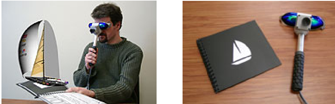
Figure 1: A tangible Augmented Reality set-up, using a book as the tangible object (Source: Mark Billinghurst, HitLabNZ, University of Canterbury, NZ)
