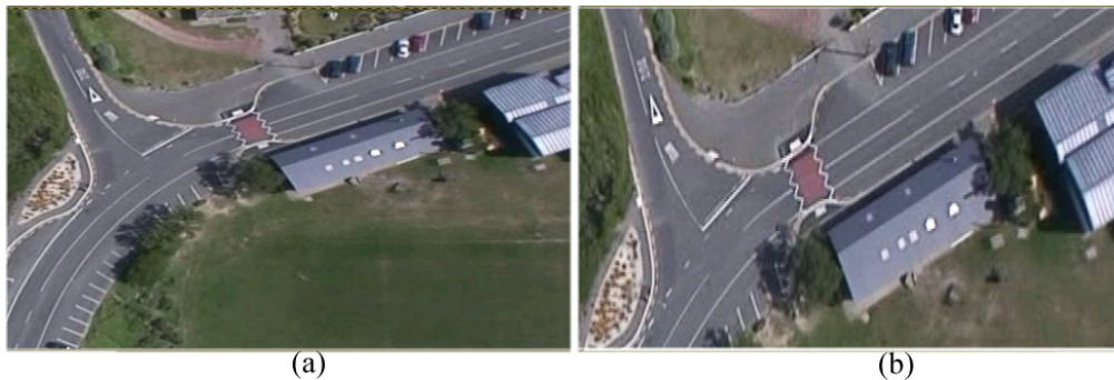
Figure 3: Pre-processed de-interlaced image (a) and re-sampled image (b). Note the distorted features (along the y-axis) in the de-interlaced image (a)
