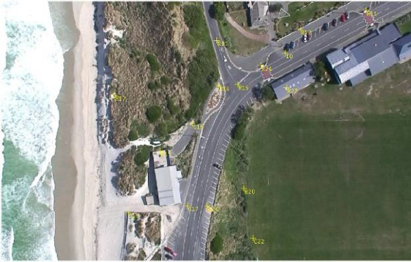
Figure 7: Aero-triangulation of the processed video-image to increase ground control over a strip of image. Note the digitized point on the roof top.
